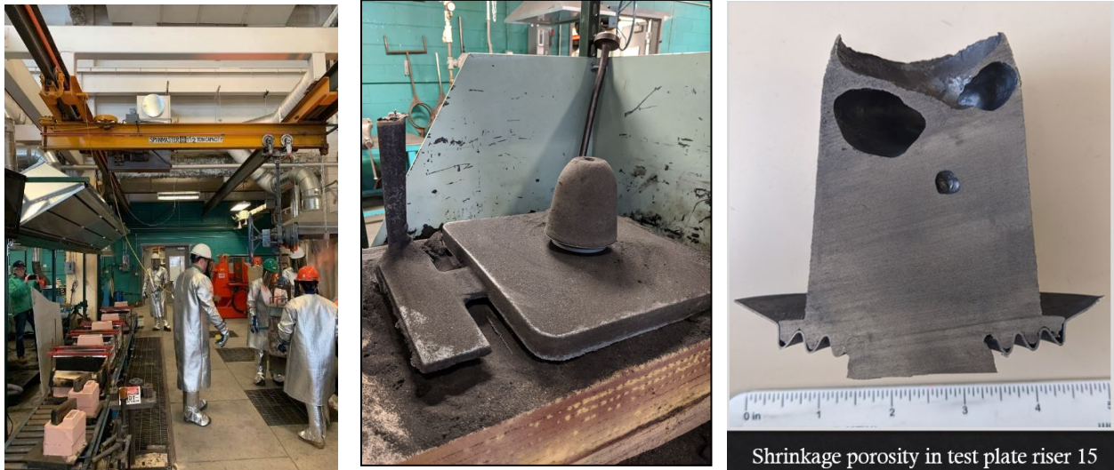
Figure 8. Test castings are poured (left view), a test plate casting with gating and sleeved riser (middle view), and shrinkage cavity in the riser (right view).
